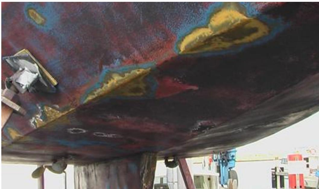
stray current leakage in a matter of just days if the current flow is high enough.
